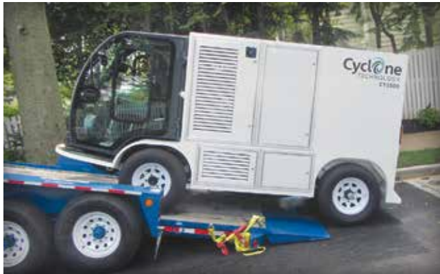
Figure 23. Equipment that provides combined power washing and vacuum
