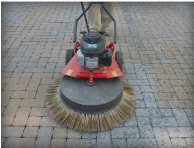
Figure 16. Rotary brushes increase cleaning efficiencies.
