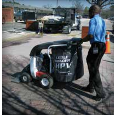
Figure 18. Walk-behind vacuum cleans a small parking area.
