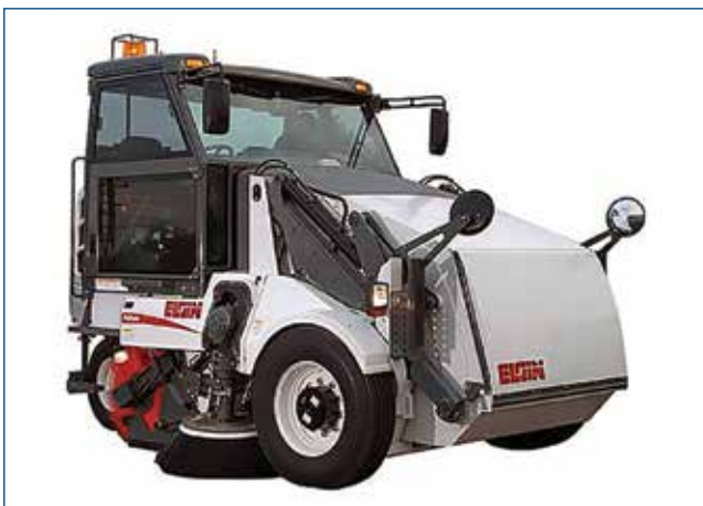
Figure 20. Mechanical sweepers use no vacuum making them the least effective of large cleaning machines.
